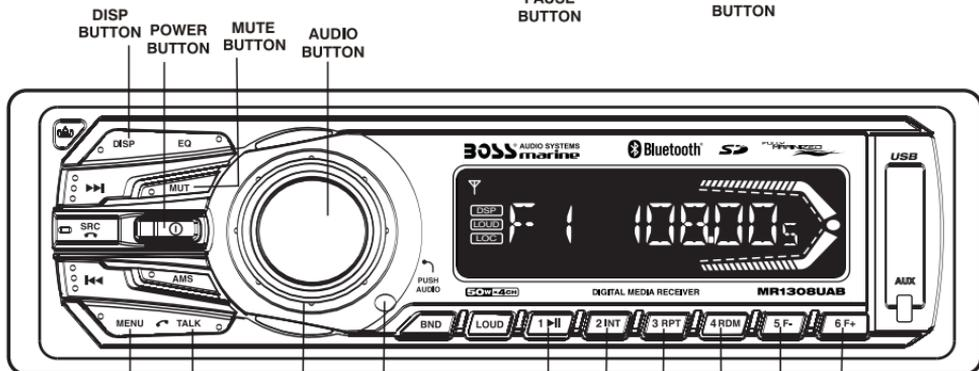
MENU BUTTON      TALK BUTTON      ENCODER VOLUME KNOB      INFRARED REMOTE SENSOR      PRESET MEMORY STATION BUTTONS (M1-M6)
